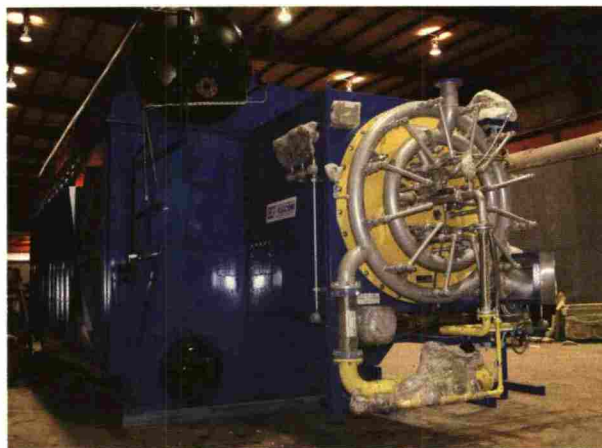
Two 75,000-lb/hr, 150-psig-output boilers can efficiently fire hydrogen, natural gas, #2 fuel oil or combinations at 20:1 turndown.
